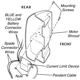
FIGURE 6 - REMOVING CURRENT LIMIT DEVICE
